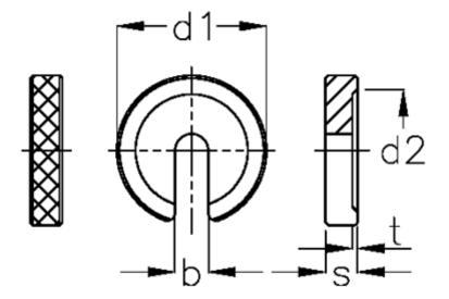
$\begin{array}{lll} b & = 6.2 \\ d1 & = 22 \\ d2 & = 16 \\ For bolt = M6 \\ s & = 6 \\ t & = 0.8 \end{array}$
